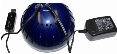
Fig. 6: Dorsal view of the device: Connection of the power supply block and the USB cable
